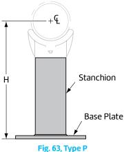
Square Cut End for use with Figure 258 or 259 Pipe Saddle Support
